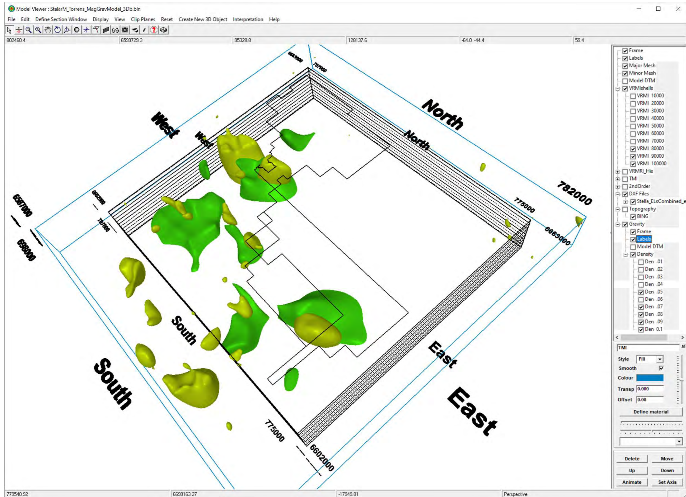
Figure 5.2: 3D Model Screen Shot Gold: Gravity Density iso-surface ( >0.05 ) Green: Magnetic susceptibility iso-surface (VRMI 0.08 SI)
